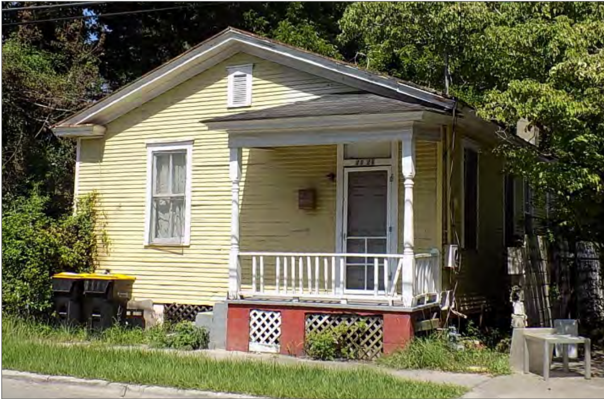
Figure 75. 2121 Harden Street (1916-20), GNAHRGIS #8379. An example of a foursquare type cottage, which has the same floorplan as a side gable cottage (two equal rooms wide, two rooms deep) but lacks a side gable roof.
