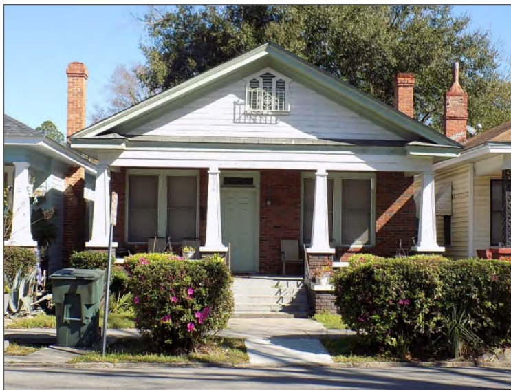
Figure 20. 628 W. 40 th Street (c1927), GNAHRGIS #8570 – This front gable bungalow is a good example of the Neoclassical Revival style as it displays the “Neoclassical cottage form” through its pedimented, temple front façade portico, tripartite gable vent, boxed gable return, and porch columns. The porch columns, however, are Craftsman style, battered wood columns resting on brick piers – a secondary stylistic element that is represented within the survey in the physical description section of GNAHRGIS and in the Survey index followed by an “(e)” which represents “elements”.
