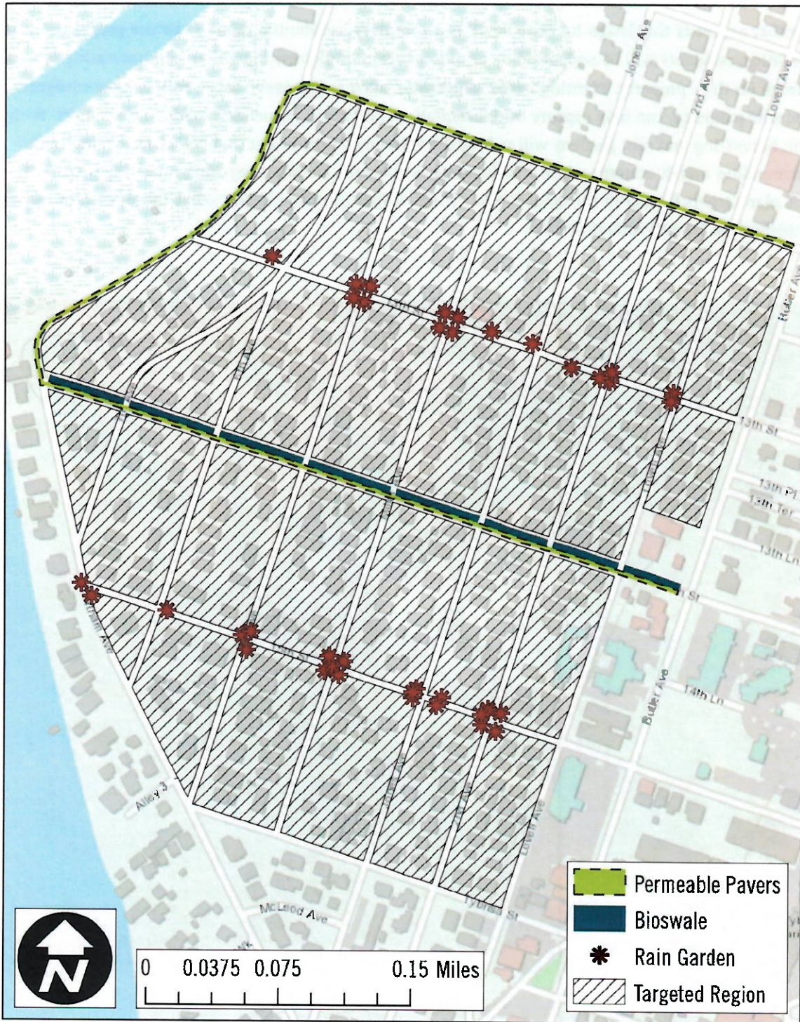
Figure 5.13. Location of proposed permeable pavers, rain storage (rain harvesting and rain gardens), and bioswale along “The Bowl.”
